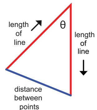
**Figure 5-4: Measure Alignment Error**
