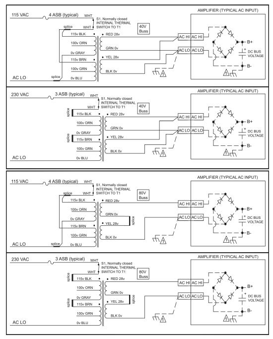
A With an isolation transformer, B- can be grounded to frame to reduce electrical noise. If B- cannont be easily accessed, the LO side of the transformer secondary should be connected to frame ground instead. DO NOT connect both the B- of the DC Bus supply and the AC LO side of the transformer secondary to frame ground at the same time.
