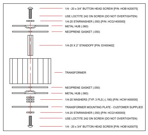
Figure 1-2: Typical Transformer Mounting
