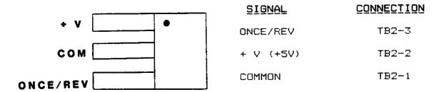
NOTE: The ONCE/REV Sensor wires must be enclosed in shielded wire with the shield connected to TB2-1 with the COMMON.
