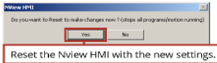
Figure 2-40: Reset to Activate Program Automation
