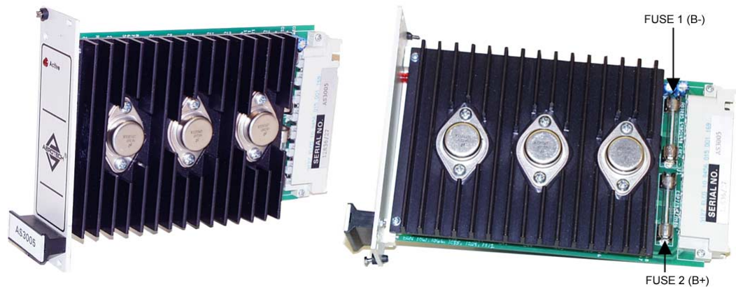
Figure 2-12. AS3005 Brushless Linear Drive Module
