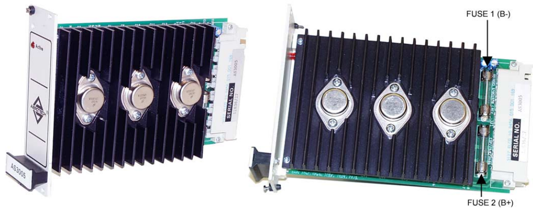
Figure 2-12. AS3005 AC Brushless Linear Drive Configuration
