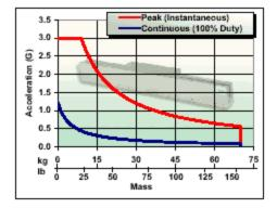
Figure 3-3: Acceleration vs. Mass for ALS20000 / ALS25000 Series Stages
