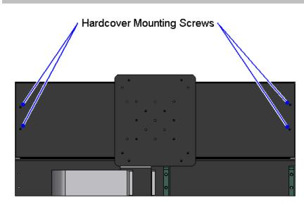
Figure 2-2: Top View of ALS20000 / ALS25000 Stage Showing Hardcover Mounting Screws
