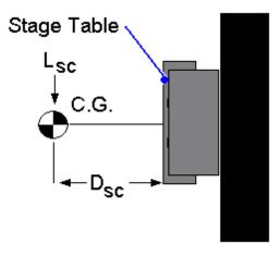
Figure 3-2: Finding L<sub>SC</sub> for Side-Mounted Stages
