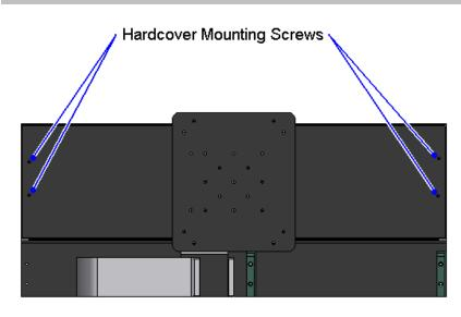
Figure 4-1: Top view of ALS20000 / ALS25000 Stage Showing Hardcover Mounting Screws
