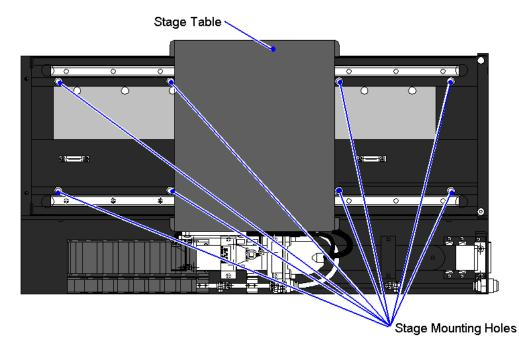
Figure 2-3: Internal View of ALS20000 / ALS25000 Stage Showing Mounting Holes
