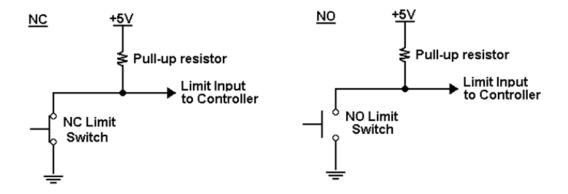
Figure 3-4: Normally Closed (NC) and Normally Open (NO) Limit Switch Wiring
