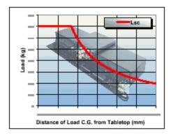
Figure 3-1: Load Capability of ALS20000 / ALS25000 Series Stages
