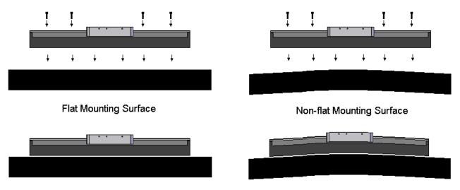
Figure 2-1: Results of Flat Versus Non-Flat Mounting
