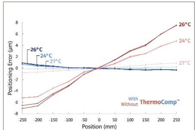
*Measurement data showing successful compensation of thermal related positioning errors at several temperatures using the ThermoComp feature. Results are typical of stage performance with and without ThermoComp.*
