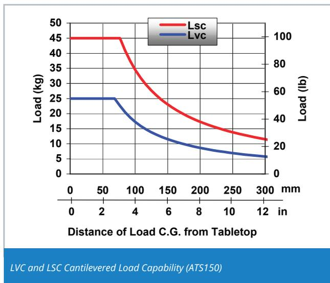
LVC and LSC Cantilevered Load Capability (ATS150)
