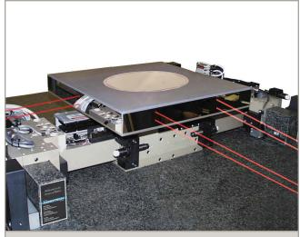
Multi-axis interferometer feedback is available to  $\textit{control}\ X$ and Y position, as well as Y-axis yaw. Use of a remote detector allows one laser source to be used for multiple axes.
