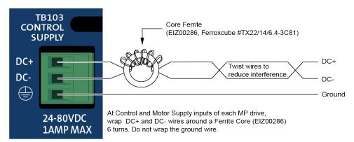
Figure 2-1: Control Supply Connections
