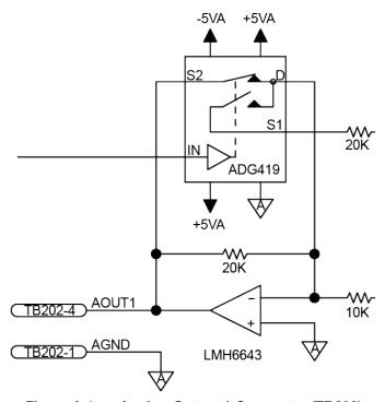
Figure 3-4: Analog Output 1 Connector (TB202)
