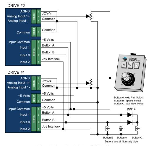
Figure 4-2: Two Axis Joystick Interface
