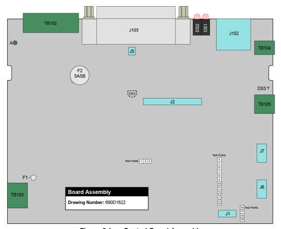
Figure 5-1: Control Board Assembly
