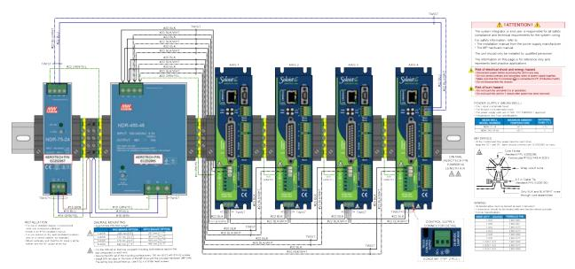
Figure 2-6: PS-MP Option (4 Axis, 480 W, 48 VDC Output, with Brake)
