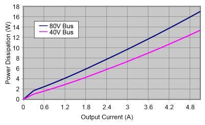
Figure 1-3: Power Dissipation vs. Output Current
