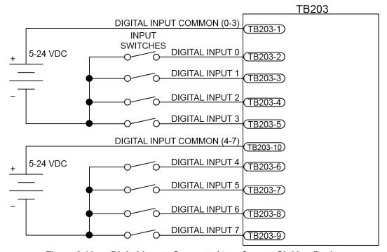
Figure 3-11: Digital Inputs Connected to a Current Sinking Device
