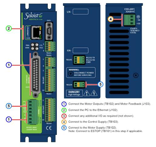
Figure 1: Quick Start Connections
