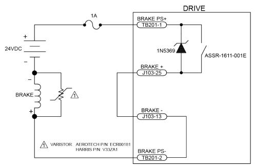
Figure 3-3: Brake Connected to TB201
