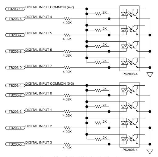
Figure 3-9: Digital Opto-Isolated Inputs
