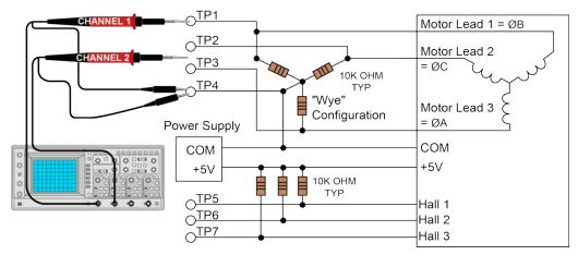
Figure 2-9: Motor Phasing Oscilloscope Example
