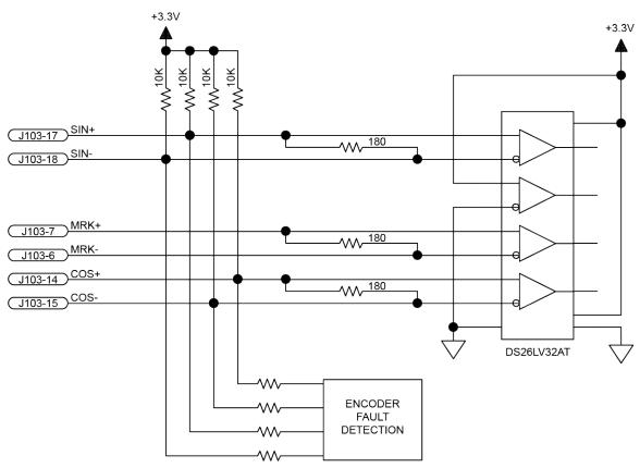
Figure 2-15: Line Driver Encoder Interface (J103)
