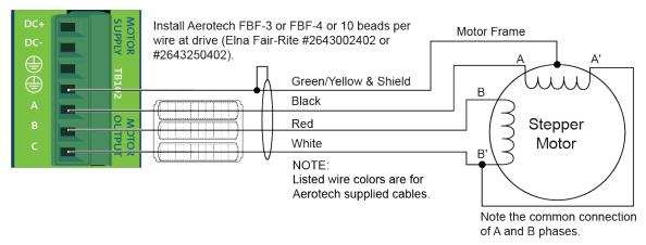
Figure 2-13: Stepper Motor Configuration
