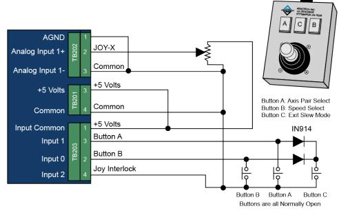
Figure 4-1: Single Axis Joystick Interface
