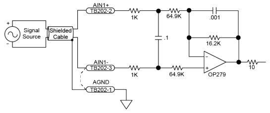
Figure 3-5: Analog Input Typical Connection (TB202)
