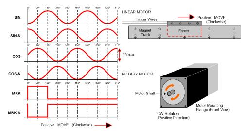
Figure 2-16: Analog Encoder Phasing Reference Diagram
