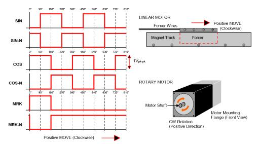
Figure 2-18: Encoder Phasing Reference Diagram (Standard)
