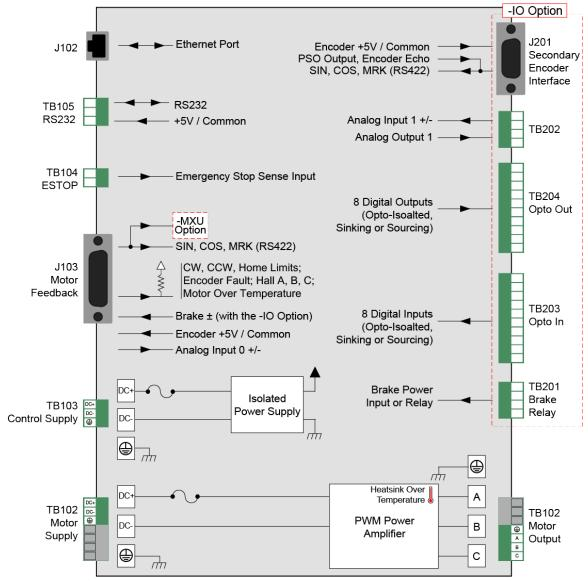
Figure 1-2: Functional Diagram
