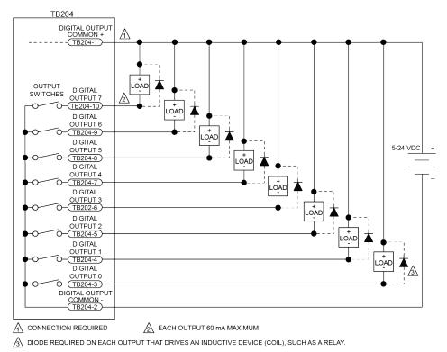
Figure 3-8: Digital Outputs Connected in Current Sinking Mode
