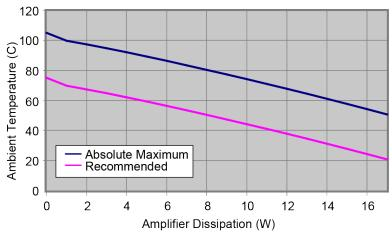
Figure 1-4: Ambient Temperature vs. Power Dissipation
