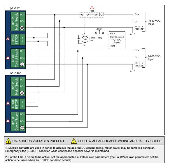
Figure 2-28: Typical Emergency Stop Circuit
