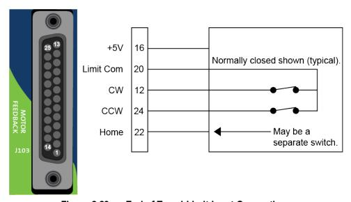
Figure 2-23: End of Travel Limit Input Connections
