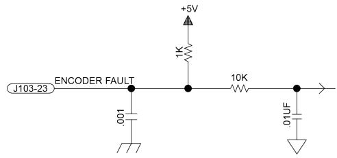
Figure 2-22: Encoder Fault Interface Input (J103)
