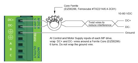
Figure 2-2: Motor Bus Input Connections
