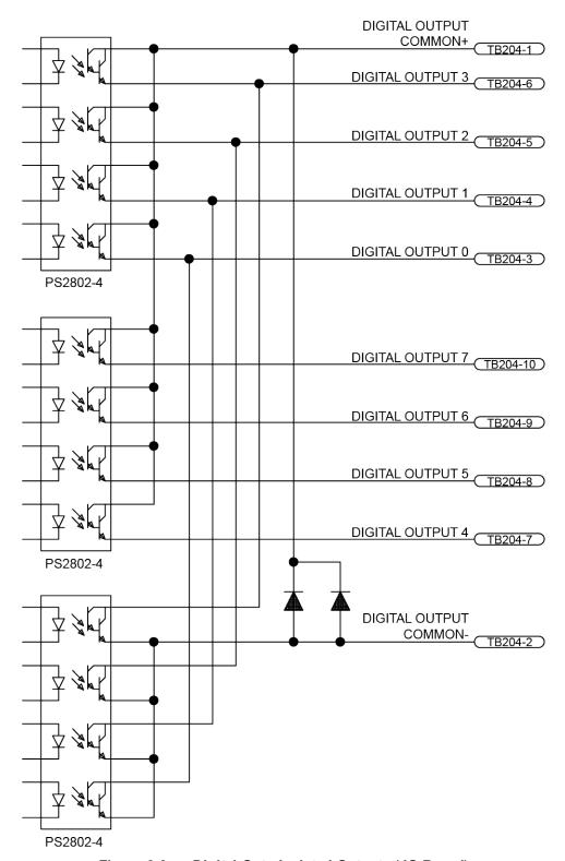
Figure 3-6: Digital Opto-Isolated Outputs (-IO Board)
