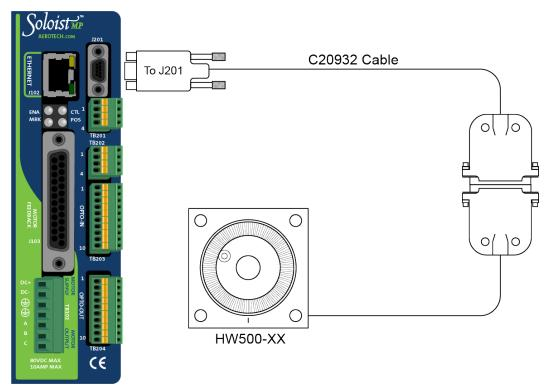
Figure 4-3: Handwheel Interconnection (to Aux I/O)
