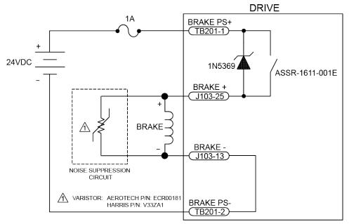
Figure 3-2: Brake Connected to J103
