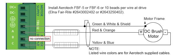
Figure 2-11: DC Brush Motor Configuration
