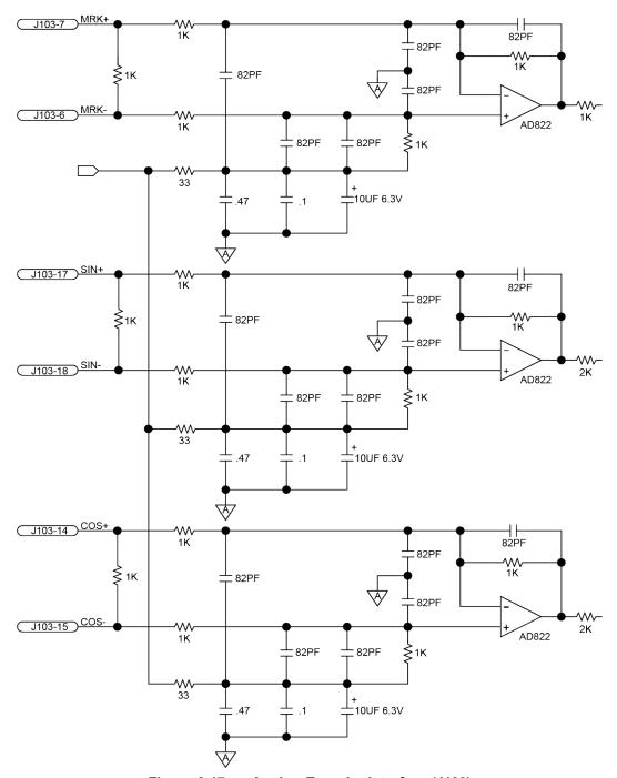
Figure 2-17: Analog Encoder Interface (J103)
