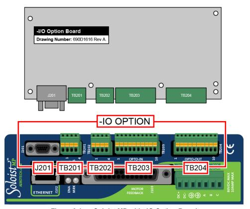
Figure 3-1: Soloist MP with -IO Option Board
