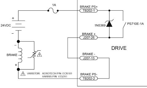
Figure 2-35: Brake Connected to TB202
