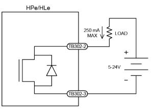
Figure 3-5: PSO Output Sinks Current
