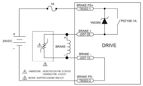
Figure 2-34: Brake Connected to J207
