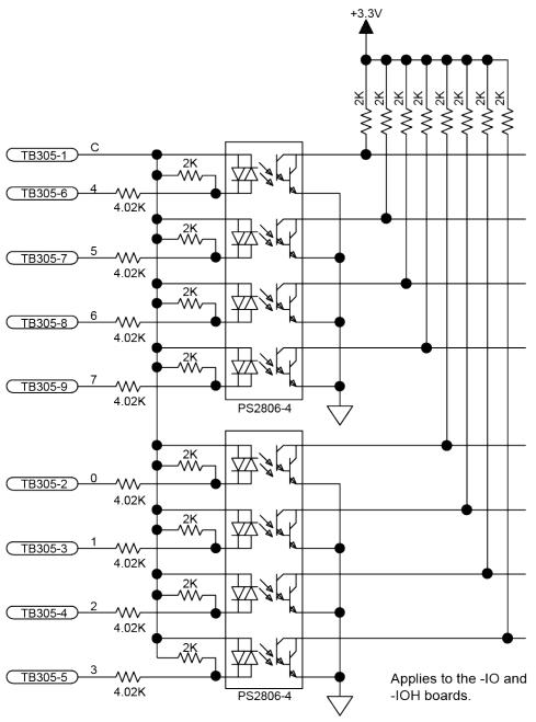
Figure 3-8: Digital Opto-Isolated Inputs
