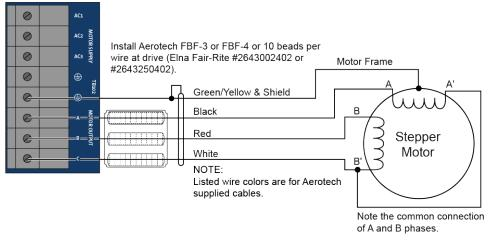
Figure 2-9: Stepper Motor Configuration
