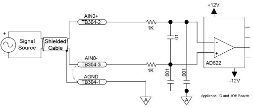
Figure 3-7: Analog Input Typical Connection (TB304)
