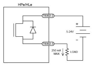
Figure 3-4: PSO Output Sources Current
