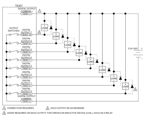
Figure 3-13: Digital Outputs Connected in Current Sinking Mode
