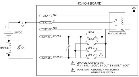
Figure 3-3: Brake Connected to TB301
