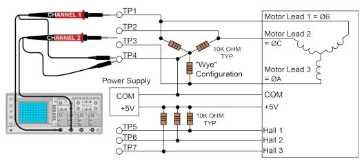
Figure 2-5: Motor Phasing Oscilloscope Example
