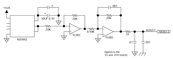
Figure 3-6: Analog Output Connector (TB303)
