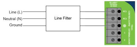
Figure 2-1: Control Supply Connections
