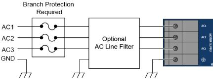
Figure 2-2: Motor Bus Input Connections
