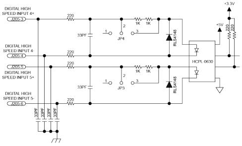
Figure 2-31: High-Speed Inputs (J205)
