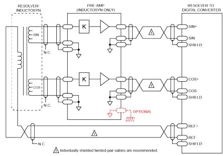
Figure 4-2: Resolver/Inductosyn Recommended Wiring
