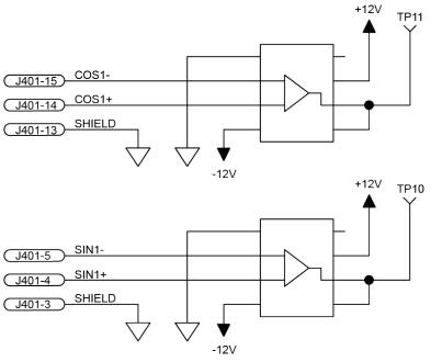
Figure 4-3: Resolver Inputs
