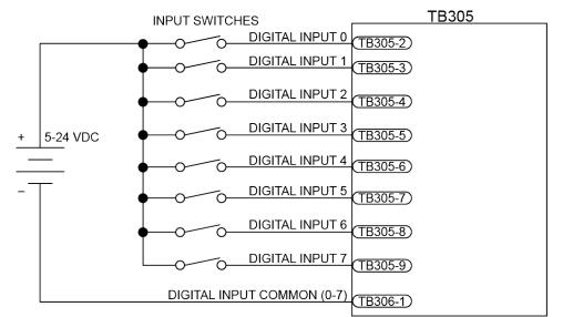
NOTE: Each bank of 8 Inputs must be connected in the all sourcing or all sinking configuration.
