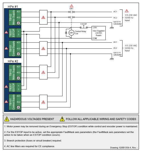
Figure 2-24: Typical Emergency Stop Circuit
