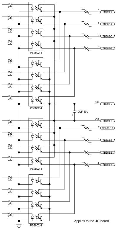
Figure 3-11: Digital Opto-Isolated Outputs (-IO Board)
