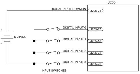
Figure 2-30: Inputs Connected in Current Sinking Mode (J205)
