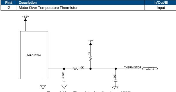
Figure 2-18: Thermistor Interface Input (J207)
