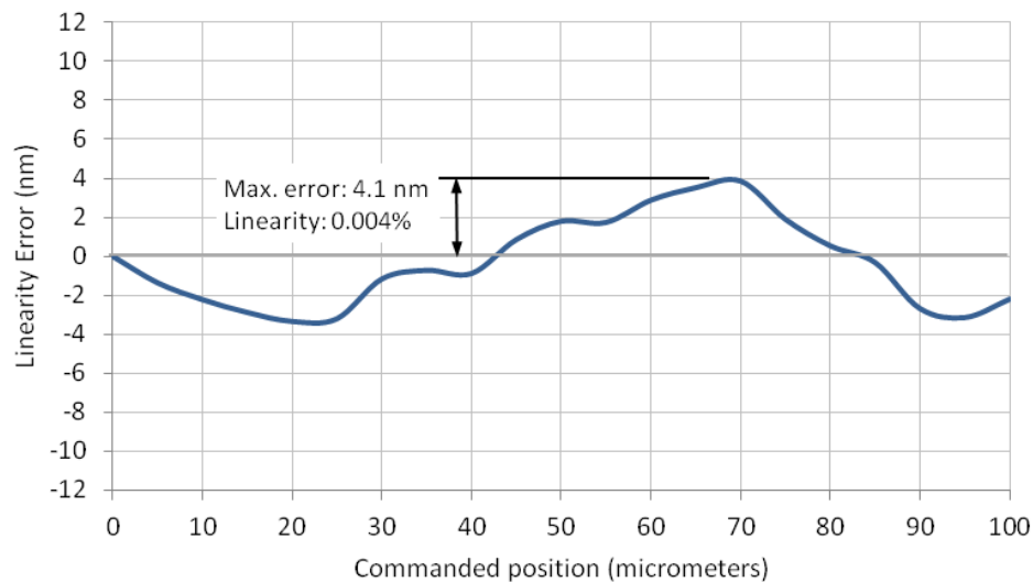
Figure C-9: Illustration showing how linearity is calculated based on measurement data taken from a 100 \mu\text{m} piezo nanopositioning stage
