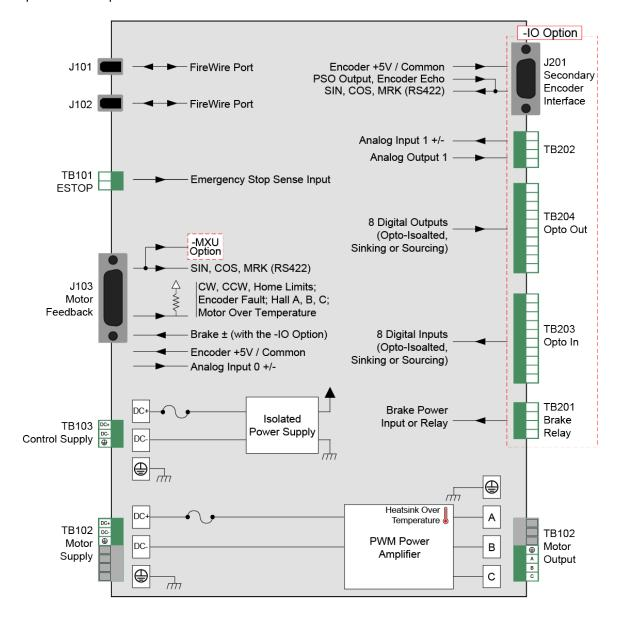
Figure 1-2: Functional Diagram
