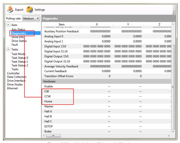
Figure 2-25: Limit Input Diagnostic Display
