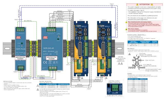
Figure 2-5: PS-MP Option (2 Axis, 240 W, 48 VDC Output, with Brake)
