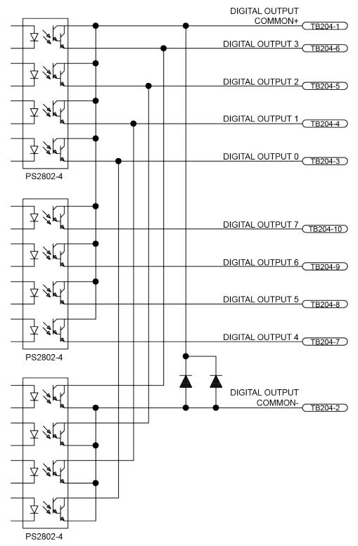
Figure 3-6: Digital Opto-Isolated Outputs (-IO Board)
