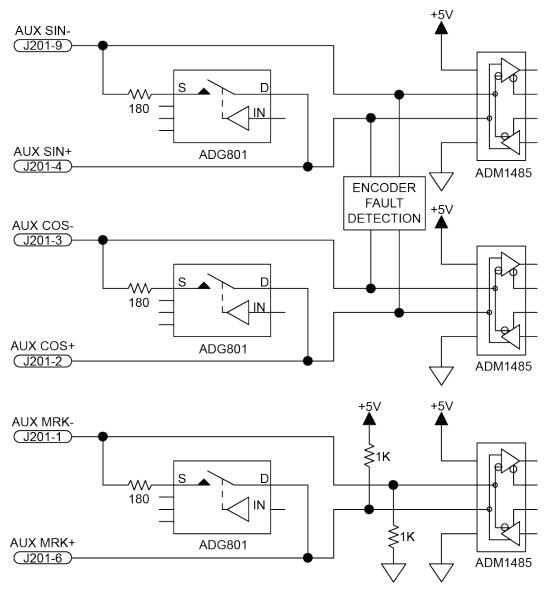
Figure 3-12: Auxiliary Encoder Channel (J201)
