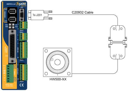
Figure 4-3: Handwheel Interconnection (to Aux I/O)
