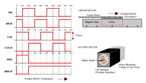
Figure 2-18: Encoder Phasing Reference Diagram (Standard)
