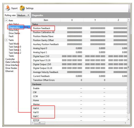
Figure 2-8: Encoder and Hall Signal Diagnostics
