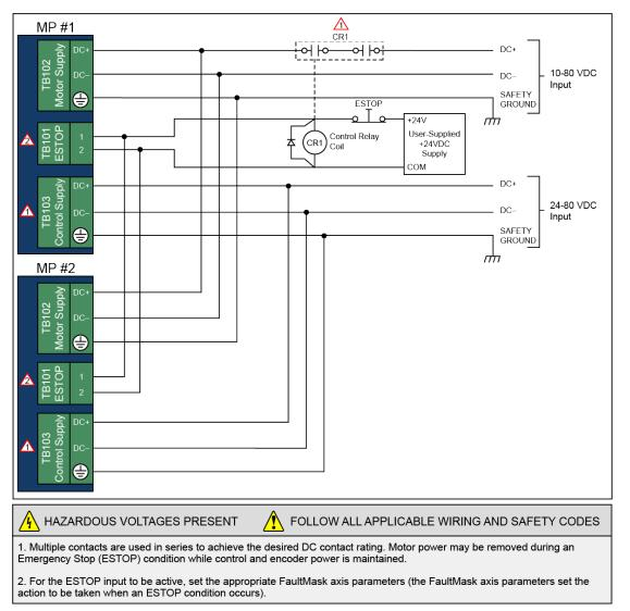
Figure 2-28: Typical Emergency Stop Circuit
