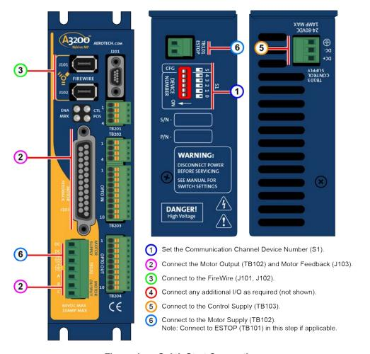
Figure 1: Quick Start Connections
