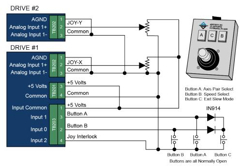
Figure 4-2: Two Axis Joystick Interface
