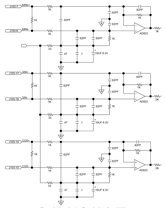
Figure 2-17: Analog Encoder Interface (J103)
