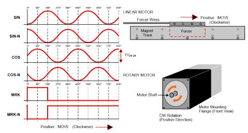
Figure 2-16: Analog Encoder Phasing Reference Diagram
