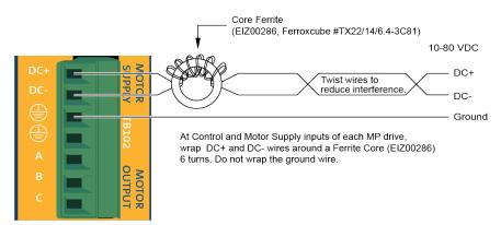
Figure 2-2: Motor Bus Input Connections
