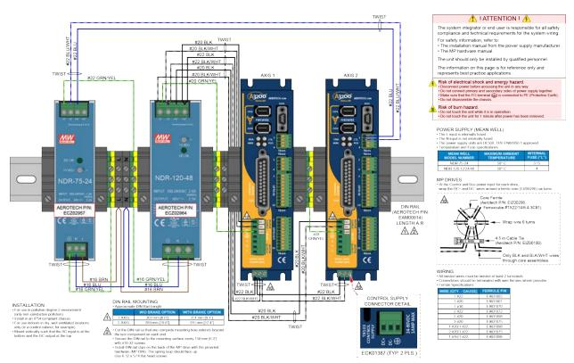
Figure 2-4: PS-MP Option (2 Axis, 120 W, 48 VDC Output, with Brake)
