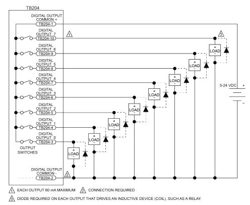
Figure 3-7: Digital Outputs Connected in Current Sourcing Mode
