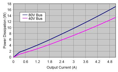
Figure 1-3: Power Dissipation vs. Output Current
