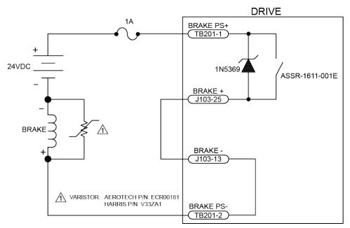
Figure 3-3: Brake Connected to TB201
