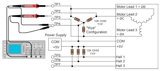
Figure 2-9: Motor Phasing Oscilloscope Example
