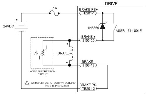
Figure 3-2: Brake Connected to J103
