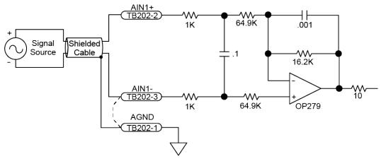
Figure 3-5: Analog Input Typical Connection (TB202)
