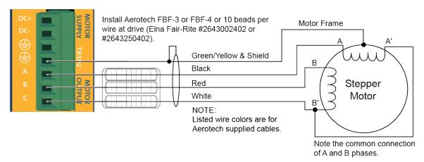
Figure 2-13: Stepper Motor Configuration
