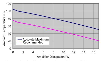
Figure 1-4: Ambient Temperature vs. Power Dissipation
