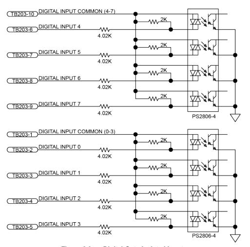
Figure 3-9: Digital Opto-Isolated Inputs
