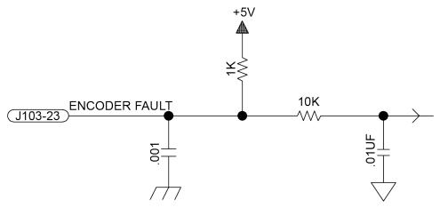
Figure 2-22: Encoder Fault Interface Input (J103)
