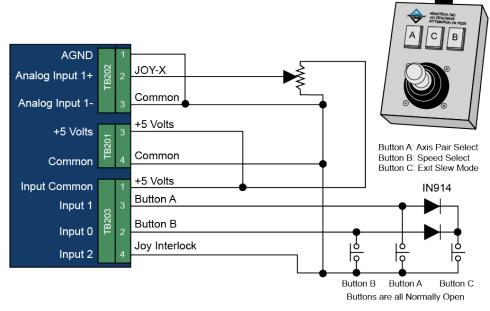
Figure 4-1: Single Axis Joystick Interface
