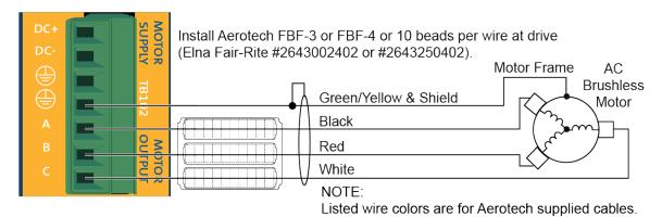
Figure 2-7: Brushless Motor Configuration
