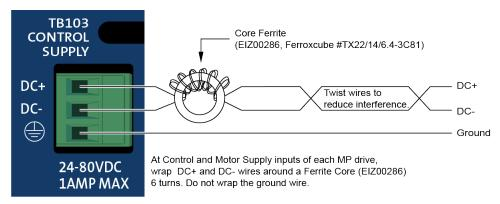
Figure 2-1: Control Supply Connections
