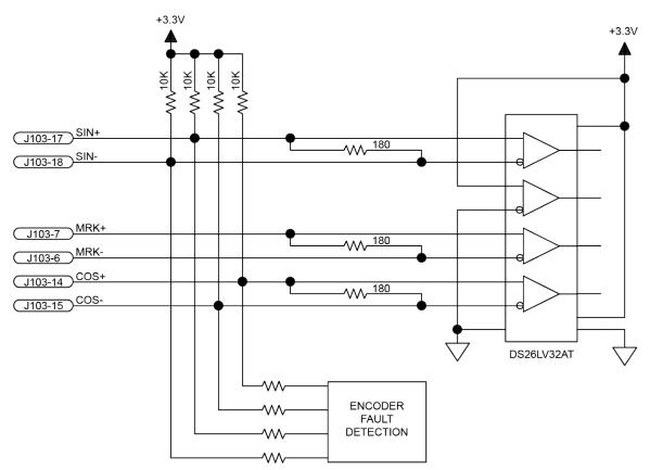
Figure 2-15: Line Driver Encoder Interface (J103)
