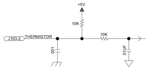
Figure 2-21: Thermistor Interface Input (J103)
