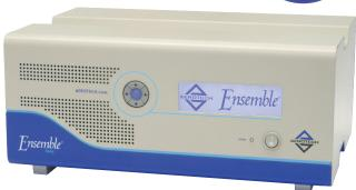
The Ensemble® Epaq is Aerotech's next-generation, stand-alone controller for moderate- to high-performance applications. It offers functionality appropriate for applications from basic laboratory experimentation and general purpose positioning to advanced OEM systems at an affordable price.
