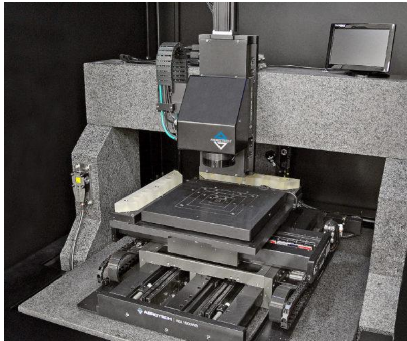
Figure 2. An image of an example precision inspection machine installed in a temperature-controlled environment. Plane mirrors are integrated into the payload plate, providing laser interferometer feedback at the work point plane for motion control.
